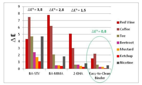
**Figure 6**. The average of  $\Delta E$  and especially the  $\Delta E$  of red wine and coffee are much lower for the paint based on the easy-to-clean binder compared to the paints based on traditional binders.
