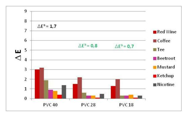
**Figure 7**. The average  $\Delta E$  at different PVC of paints based on the easy-to-clean binder. The gloss at 60° for the PVC 40 paint is 15, for the PVC 28 paint 24 and for the PVC 18 paint 80. The effect of PVC on the stain removal properties will be investigated in more detail in the near future.
