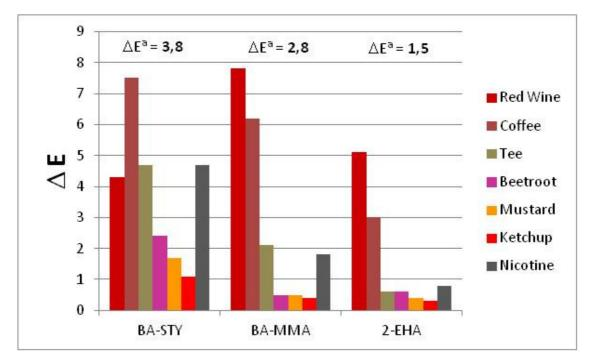
**Figure 3**. Comparison of different polymer binders in a PVC 28 paint with  $\Delta E$  indicating the stain removal performance for different house hold stains.  $\Delta E^{a}$  is the average  $\Delta E$  value of the water soluble stains.
