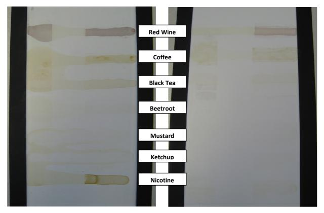
**Figure 2**. Paint films exposed to water soluble stains for 1 hour and then immediately subjected to 100 scrub cycles. A paint based on the styrene acrylic binder is shown to the left and a paint based on the acrylic binder containing 2-ethyl hexyl acrylate to the right. A problem with the styrene acrylic based paint was that the stains were floating out and connected.
