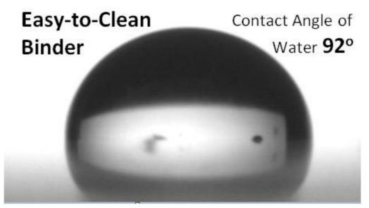
Figure 5. The contact angle of water on the polymer film of the easy-to-clean binder is 92°.
